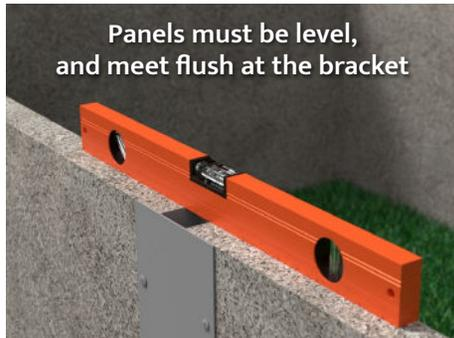
**NOTE: Sight down the walls of your GreenBed™ to make sure that the sidewalls form a straight line.** Move the side panels or the end panel until they look straight.
