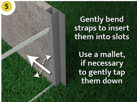
Now, install the included metal straps between each joiner bracket. Gently bend the straps, as needed, to insert them into the slots. This will keep the sides of your raised bed from spreading during installation and later when you fill it with soil.
