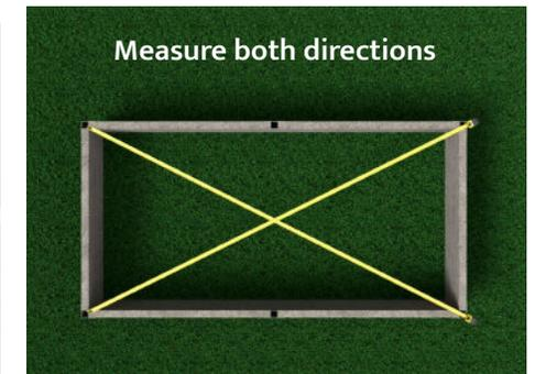
**Check your finished bed for squareness by measuring both directions diagonally.** Dimensions should be within 3/8" of each other. Adjust panels as necessary to square it up.
