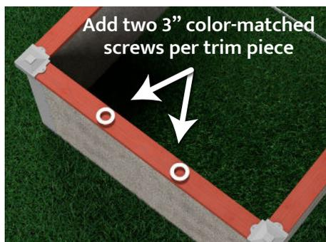
Finish securing each trim piece with two additional **color-matched, 3" screws** in the predrilled holes.
