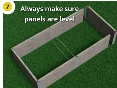
Now, install the final end panel with the pre-installed corners to complete the bed. Check that the end panel is level, and adjust the side walls so they meet evenly with the corners of the end panel. Use 1-1/2" screws to secure the corner brackets to the side panels.
